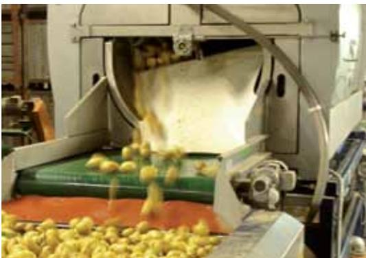
Washed and 'polished' potatoes exit this machine at the rate of 15 tonnes per hour.
