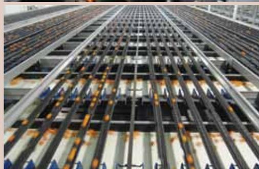
(Upper photo) In California a bank of high speed grading machines micro weigh and photo stitch analyse mandarins for blemishes across 40 lanes at 10 fruit per second per lane, and (lower photo) travel at high speed to assigned packing stations. PHOTO: WWW.COMPACSORT.COM
